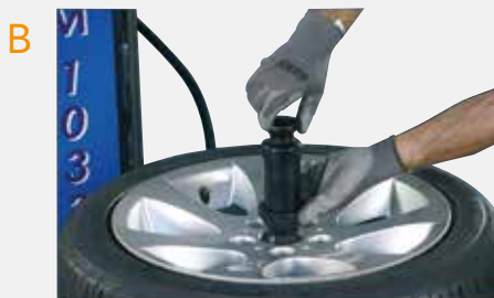
POSITIONING HANDLE WITH CONE ON THE RIM
