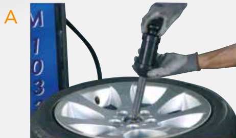
INSERT THE HANDLE WITH THE CLAMPING CONE
